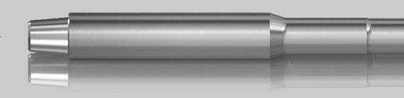
Non-magnetic drill collars were developed to allow magnetic surveying of the well trajectory using instruments inside the drill string.
