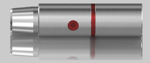
The valve is mounted on the mud motor's top sub. If there is no pressure difference between the drill string and tubing annulus during mud motor's round trip, the valve piston is hold in the upper position by spring power and the interior of the string communicates with tubing annulus via valve's hole pattern (the valve is open). During run-in-hole stage the drillstem is filled with annulus mud. When running out the mud goes to tubing annulus.
