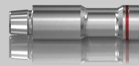
Oscillator is designed to generate low-amplitude axial oscillations in the drill string and to decrease the downhole friction. As a result it improves transmission of WOB and decreases directional stress especially during directional drilling.
